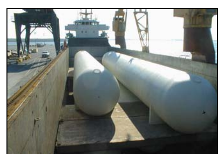
TWO TANKS SECURED ON PONTOONS
