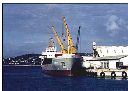
TANKS DISCHARGED WITH SHIP'S GEAR
